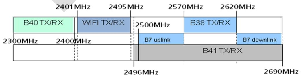
The two systems interfere with each other because of non-linear characteristic of LTE Band 38/40/41 and Wi-Fi transmitter. The main impacts are as follows:
