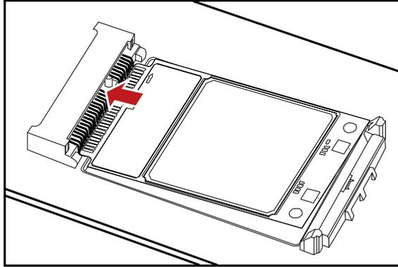
Step 2 Press downwards to fix the Mini PCIe Adapter in the module slot.
