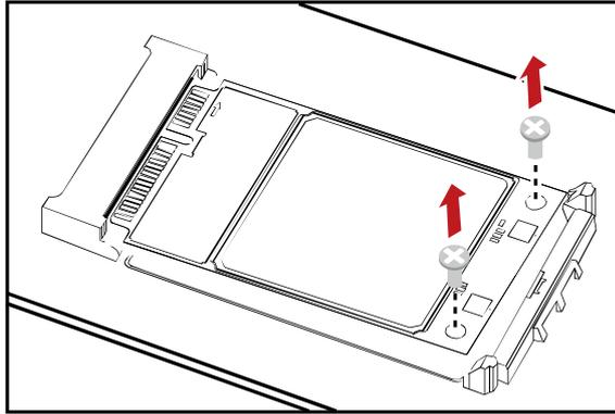
Step 3 Slide backwards the two clips to release the Mini PCIe Adapter from the slot. Then, lift up the Mini PCIe Adapter.
