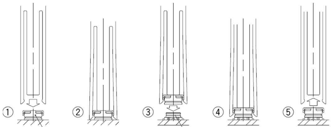
1. Align the mating tool or the mating end of the tool over the plug end of the cable assembly.
