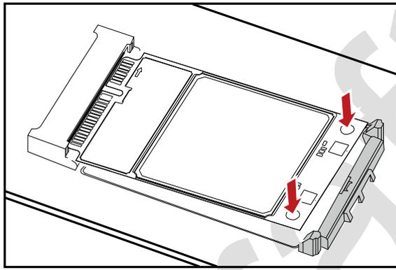
Step 3 Use a screwdriver to fix the Mini PCIe Adapter on the main board with two screws provided in the Mini PCIe Adapter packing box.
