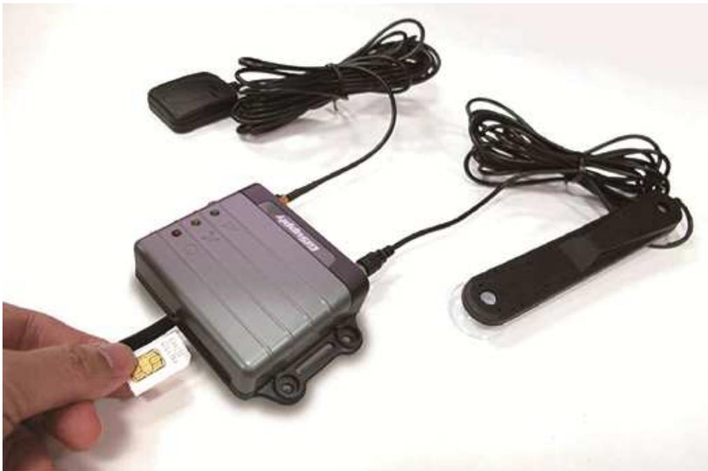
With the copper contacts facing up, align the notch on the SIM card with the notch on the SIM slot and insert the SIM card. If SIM is inserted correctly, you will not be able to see the copper contacts after inserting the card. To eject SIM card, simply, use your finger nail and apply slight pressure.
