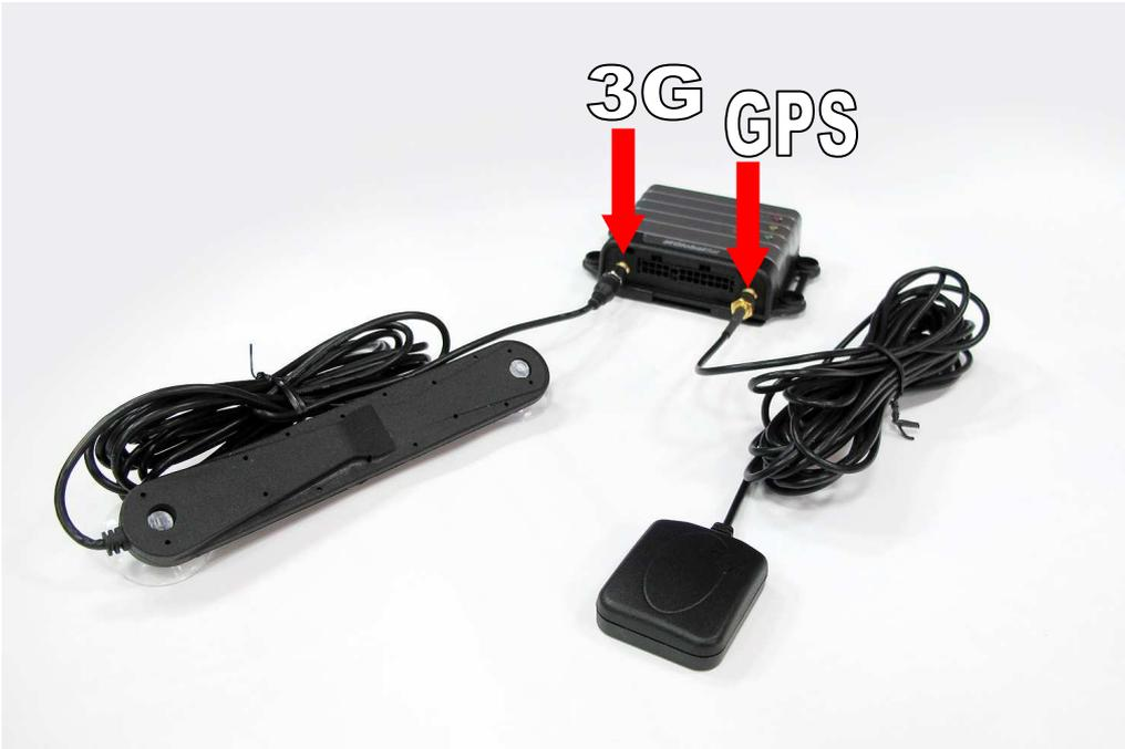
Install the 3G antenna to the 3G antenna port on the left side of the front of the device. Install the GPS antenna to the GPS antenna port on the right side of the front of the device.
